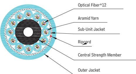
Primary Coded Fiber (250μm)
