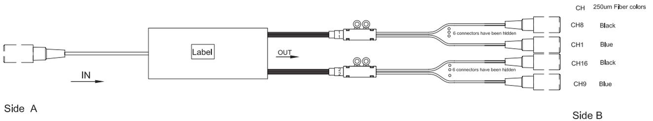
**EXAMPLE** Splitter Assembly, 2x 16 PLC Splitter
