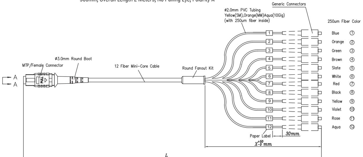
Optec's MPO/MTP® Loopback offered in female design with an economical solution provides a stable and convenient means for network testing and diagnostics.
